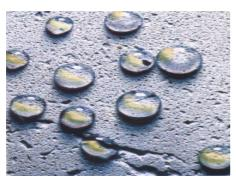
ISONEM MS 80 is a one component, transparent, penetrating silane/siloxane hydrophobic impregnant. The product reacts chemically with a mineral substrate to form a surface that is repellent to water yet still permeable to water vapour. ISONEM MS 80 protects and preserves the substrate without altering the natural surface texture or colour and without forming a film layer on the exterior surfaces where it has been applied.
