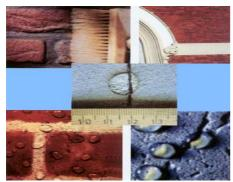
The ISONEM MS 80 molecules are very small and highly mobile. The relatively slow solvent evaporation rate allows it to enter even the smallest pores. Its water vapour permeability allows the surface to "breath" naturally. The application of ISONEM MS 80 greatly extends the life and colour retention of brick- work.
